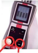
aux button: choose display damping (absolute mode) or resolution (differential mode) depending on measuring mode
